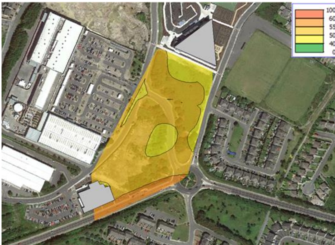
Figure 10-6 Initial Noise Risk Assessment – Night time (4m height)
