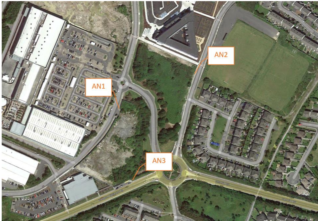
Figure 10-2 Noise Survey Locations
